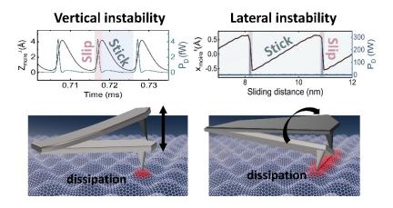
Figure 1. Moiré energy dissipation originates from vertical and lateral instability.
